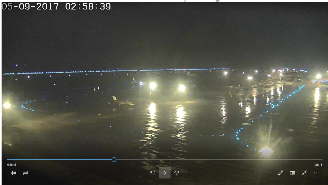
Green Centreline light extending upto the taxi track link Taxiway F. Review of ATC tape reveals, no request was made by VT-AYB for increasing the intensity of lights
